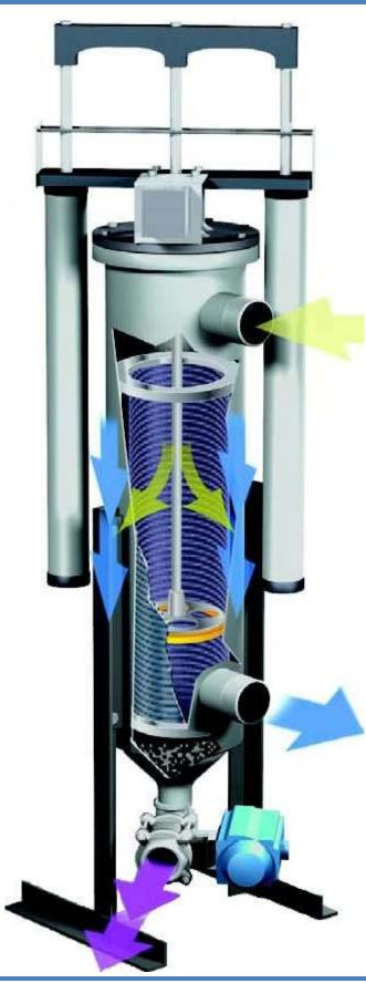
too large to pass thorough the element end-up falling to the bottom of the vessel or become stuck against the inner circumference of the element wall.
