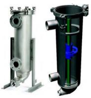
The functionality of the MCF-824 is the same as the other DCF automatic filter systems with the difference being there is a hollow shaft at the center of the system containing a magnet which is coupled to an external magnet attached to the cleaning disc. Pneumatic actuation from standard shop compressed air injected through the base of the center column pushes the internal magnet up and down. The outer magnet within the cleaning disc follows the internal magnet.
